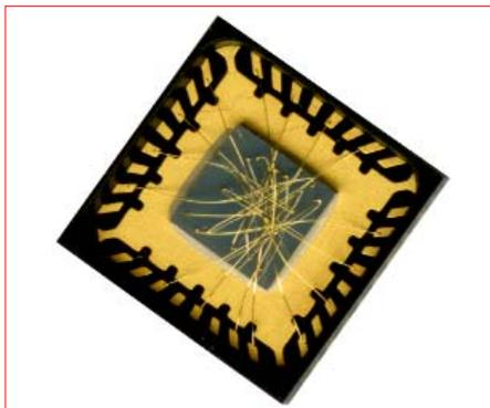
*The X-Wires can be seen in this Mirror Semiconductor open-cavity QFN package prototype.*
