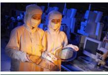
Technicians at a STATS ChipPAC plant inspect a wafer prior to assembly.
