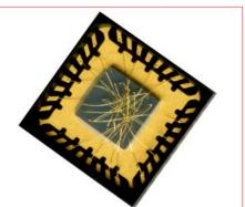
Semiconductor open-cavity QFN package prototype.
